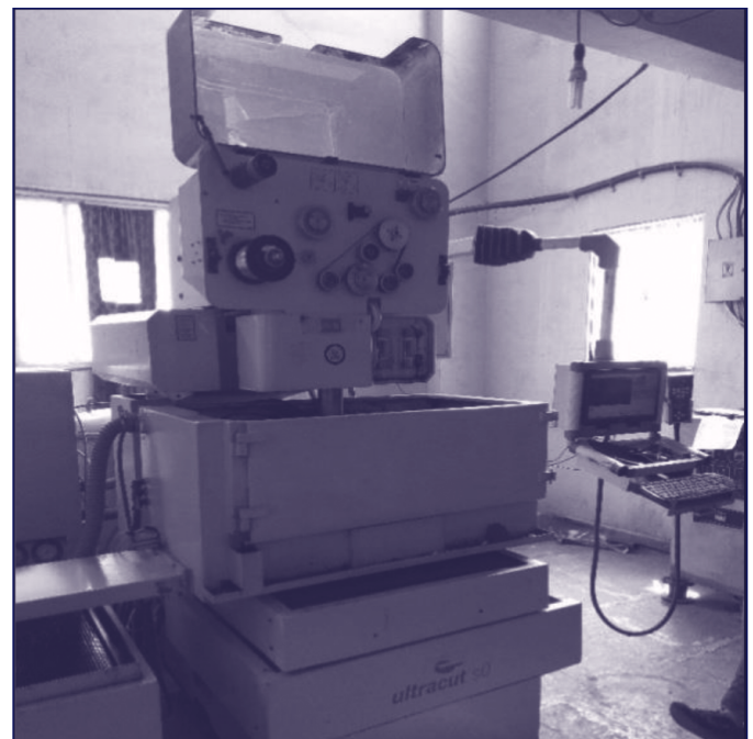
Fig. 2. WEDM experimental for processing Al/Gr/Cp MMC.
